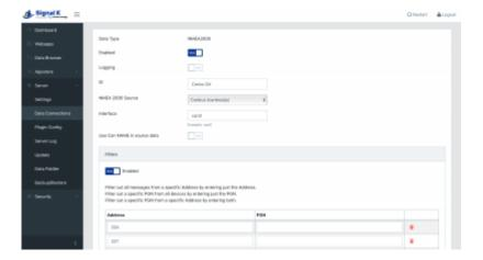
Note that, to keep that operational, that port must be configured as a 250kbit VE.Can & NMEA2000
