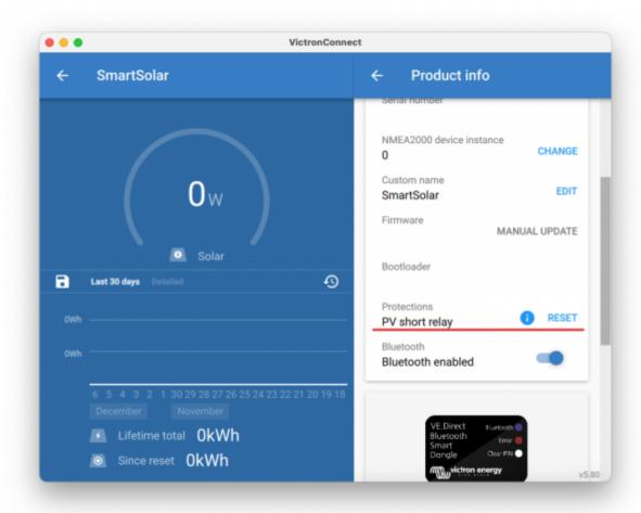
Note that the feature only shows when (a) the connected units features the protection, ie. 250/100 VE.Can model, HQ2150 and later; (b) requires the battery voltage to be between 10 and 15V; (c) requires VictronConnect v.580 or later; (d) requires firmware version v3.12 or later to be installed on the Solar Charger and (e) no error 80 to 83 is active.
